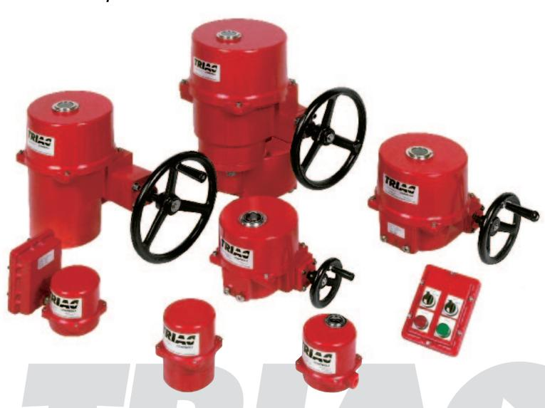
Triac Controls line of electric actuators offers a broad range of torques from 300 to 30,000 in. lbs. and numerous features including manual overrides, auxiliary switches, 4-20ma modulating control, several voltage options including 1-phase 24/120V/220V - 12 and 24VDC, 3-phase 220v, 380v, and 440v. The units feature EPI-CYCLICAL gear trains and a unique manual override with handwheel.
